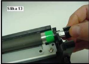
Well all 3 have one thing in common—they work on same principle. They all work with triboelectric friction between surface of developer roller and doctor blade. This energy is better expressed if surface of developer roller and db is rough.
